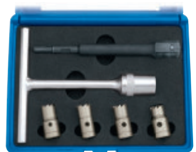
Diesel Injector Seat Cutter Set (6 Piece)
